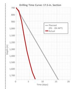
The above graph compares the actual time (red) and the planned time (gray) to drill the 17.5-in. hole section. The Magnus RSS reached section TD in only 7 days.
